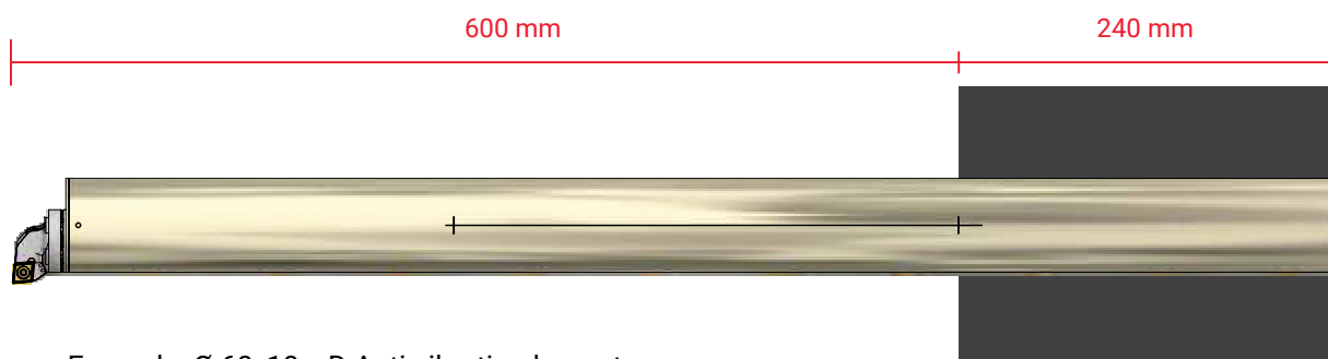
Example: Ø 60, 10 x D Anti-vibration bar setup
